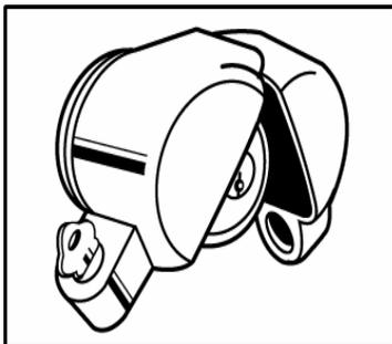
Clam shell locks are designed to prevent use of the door or occupant's keys to unlock entrance doors.
