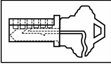
Key-way locks are designed to prevent use of the occupant's keys to unlock entrance doors. These function by inserting a two-part locking key into the door keyhole and removing only half of the key. The other half of the locking key remaining in the door prevents insertion of the occupant's key.
